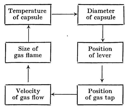
The reader should verify that each arrow represents a physical action which can be demonstrated if all variables other than the pair are kept constant.' 6
